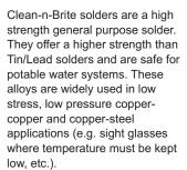
Clean-n-Brite is a Lead-free, silver-bearing high-strength solder used for applications requiring close joint clearances.
